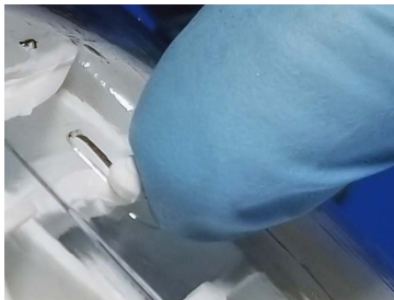
3. Push the top of the Mounting Post all the way to the back of the narrow end of the Mounting Slot.
